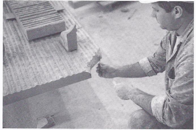
2 Mixed epoxy glue is spread thinly on both faces. Keep glue away from face edges as much as possible to avoid squeeze-out.
